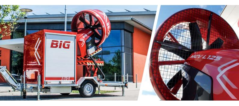
The MGV<sup>®</sup> L125 is extreme powerful and allows an effective ventilation of large industrial facilities, underground parking, high-rise buildings, airports, shopping centres or miles long tunnels – in tests at traffic tunnels, an air output up to 1.000.000 m<sup>3</sup>/h had been measured. This ventilator with its powerful, reliable car engine is the ideal partner for every fire service who has to deal with fires or dangerous incidents in large structures.
