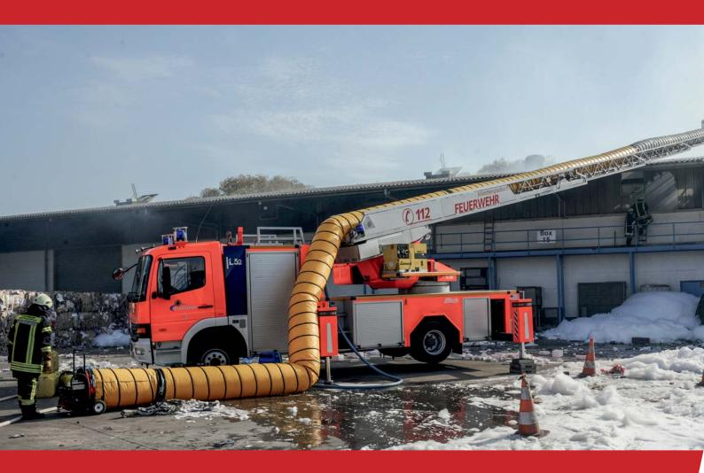
The FlexiFoam system is ideal for operations when rooms have to be flooded or greater areas have to be covered with foam.
