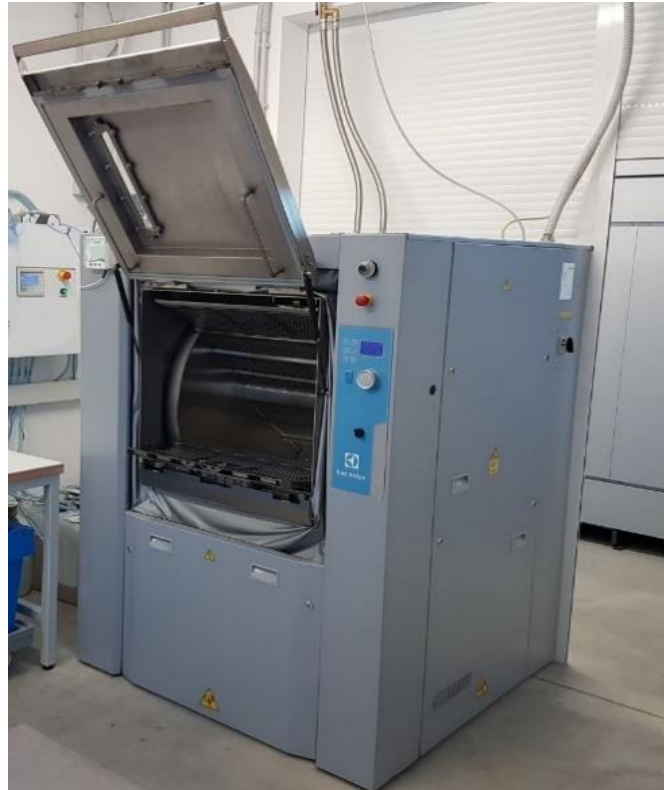
Picture 11 and 12. Examples of barrier washing machines that can be programmed with the Lejon Kemi washing program for breathing masks with or without disinfection steps.
