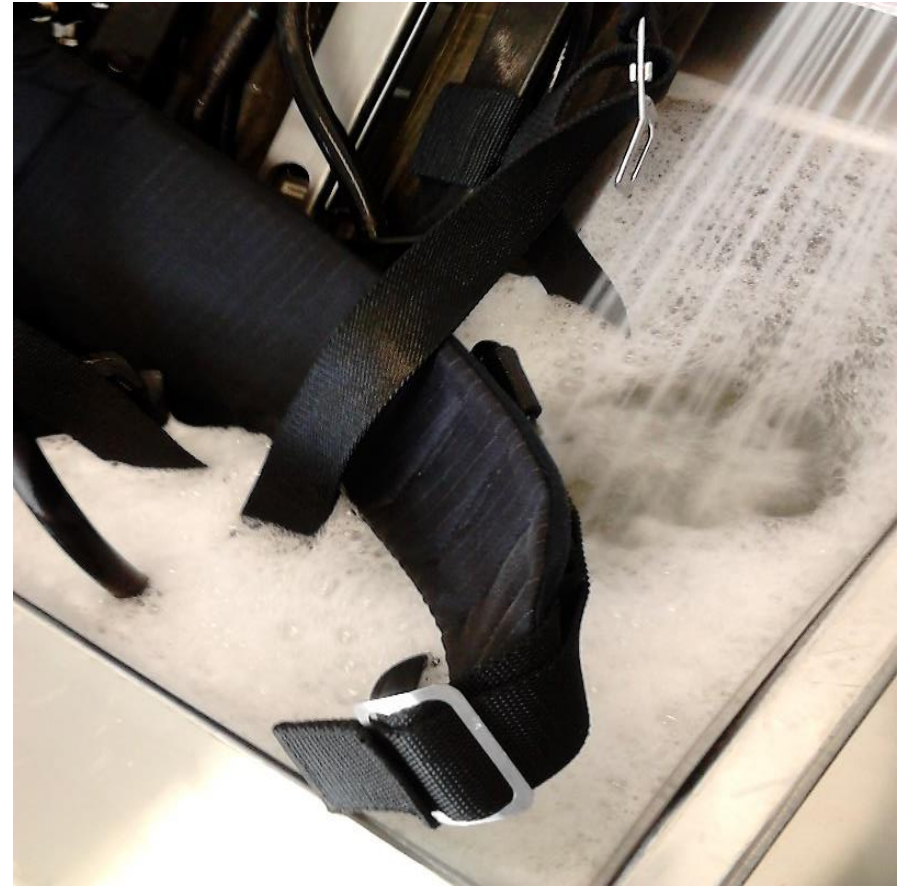
Picture 8. Residues after foaming detergents can cause excessive foaming inside a PPE-dishwasher
