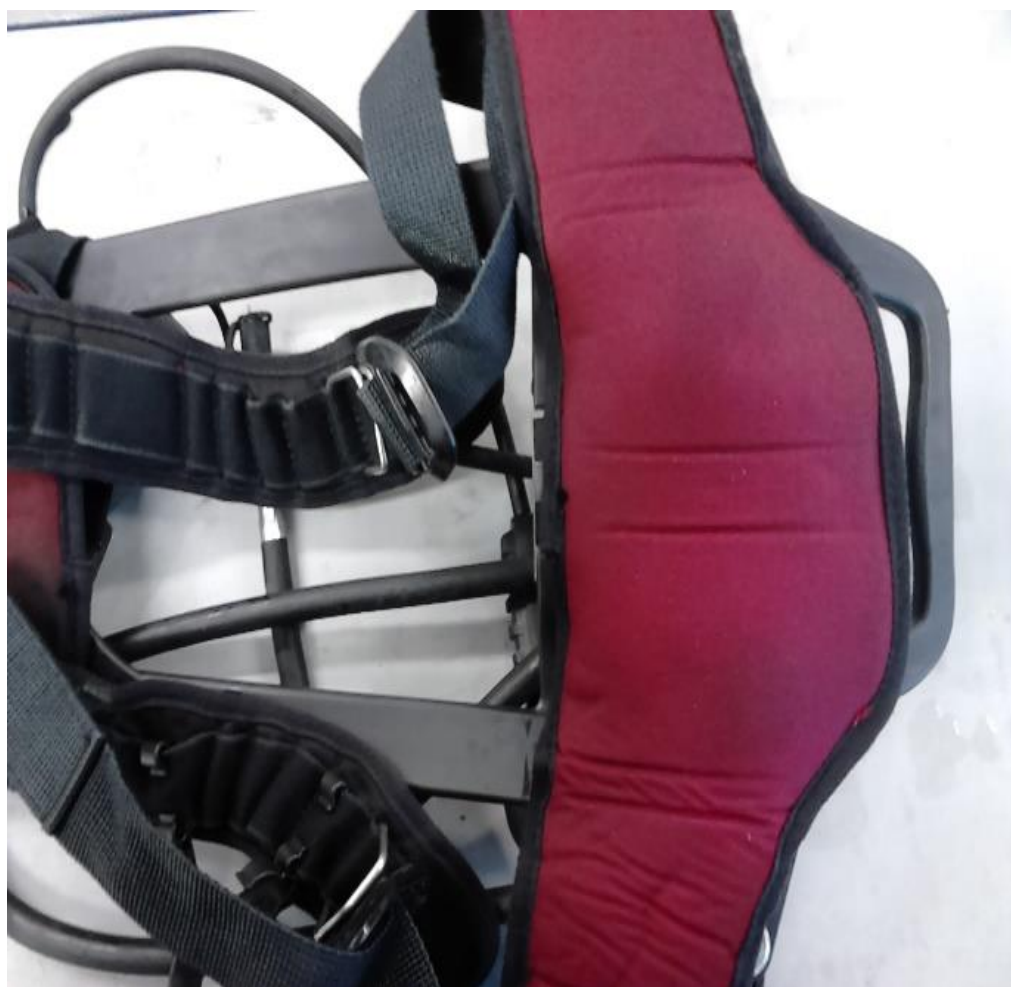
Figure 10. Breathing apparatus after pretreatment with concentrated FFE Cleaner, which was sprayed on and allowed to act for about 3 minutes before cleaning in PPE-dishwasher for 20 minutes at 60° C, with 1 % FFE Cleaner.
