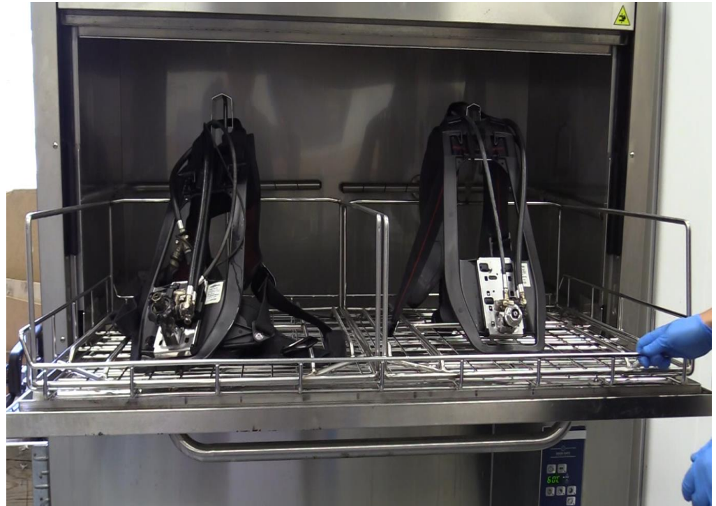
Picture 6. Carrier racks for breathing apparatus after pretreatment in a PPE-dishwasher from Electrolux Professional AB
