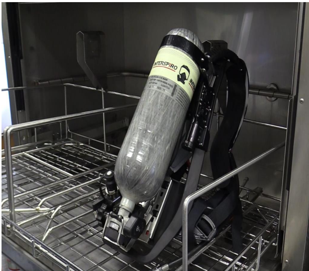
Picture 9. Breathing apparatus after pretreatment with concentrated FFE Cleaner, which was sprayed on and allowed to act for about 3 minutes before cleaning in a PPE-dishwasher for 20 minutes at 60° C and with 1 % FFE Cleaner.
