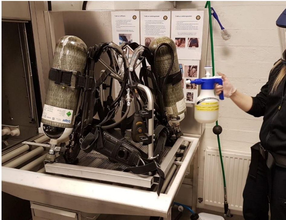
Picture 5. Breathing apparatus is pretreated before washing in PPE-dishwasher of “barrier model” from Wexiödisk AB
