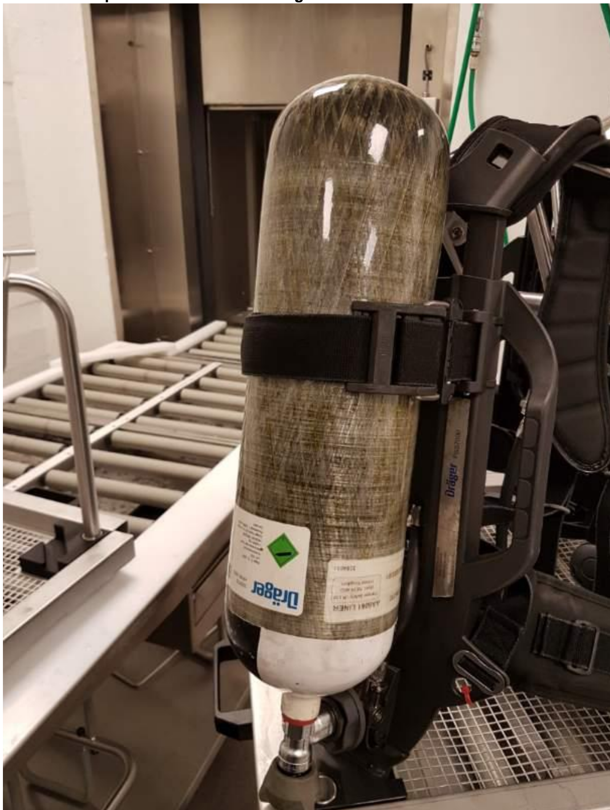
Image 3. Air cylinder and carrying strap after pre-treatment with concentrated FFE Cleaner followed by washing in a PPE dishwasher at 60 °C for 20 minutes with 2 % FFE Cleaner. The cleaning result was excellent according to visual assessment and according to analyses of 16 different PAHs before and after cleaning.
