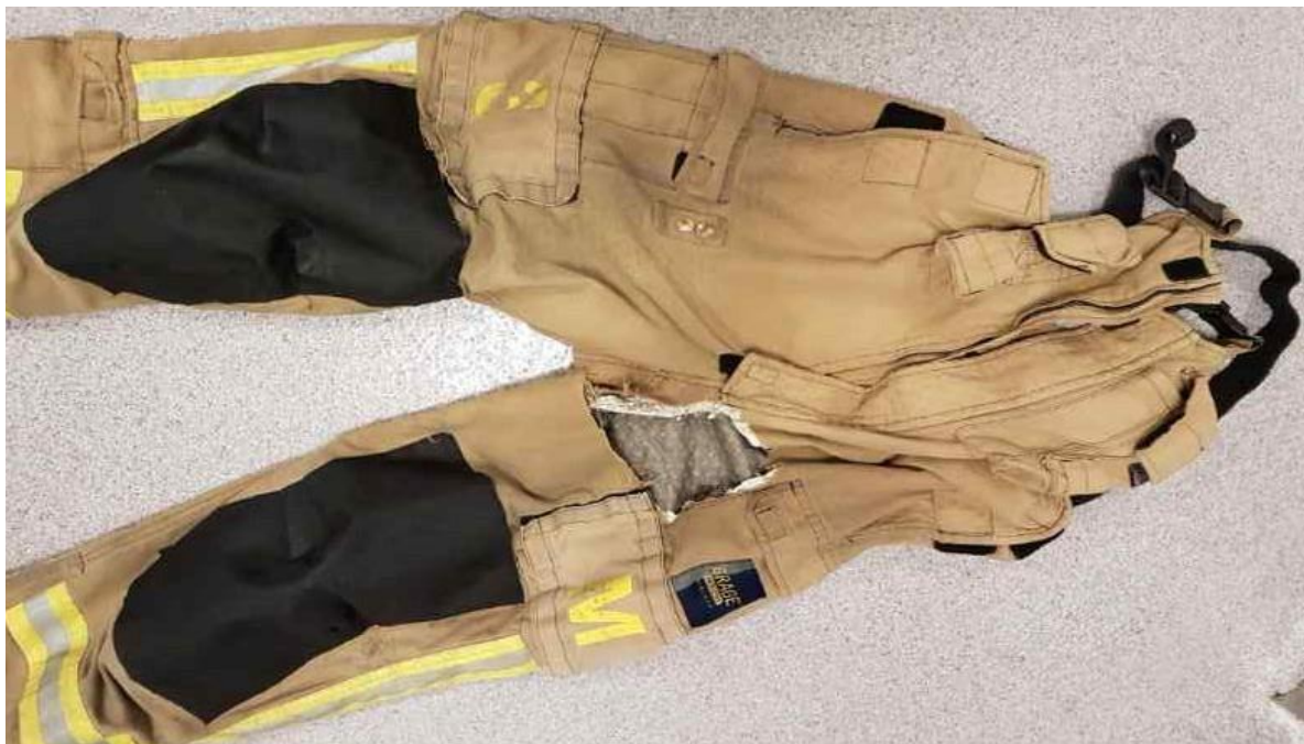
Photo 4. Picture of washed turn out gear (trousers) from which a sample has been taken for analysis of PAHs.
