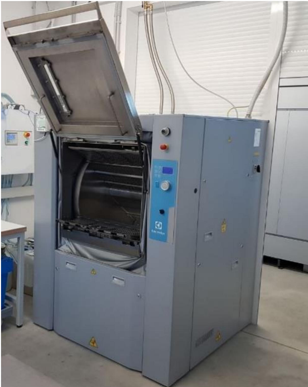
Photo 2. Barrier washing machine in fire station with contaminated zone and clean zone division for handling of, for example, emergency suits and breathing masks.
