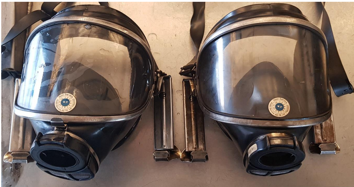
Picture 3. Breathing mask on the left side is cleaned with Lejon Kemi detergent FPG Wash in a washing machine with washing bags and washing program developed by Lejon Kemi and the breathing mask on the right side is cleaned with an ordinary machine dishwashing agent during 6 minutes in a PPE dishwasher at 50° C.
