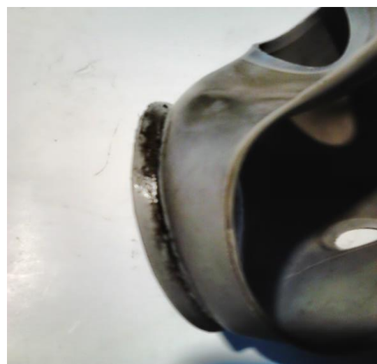
Images 1 and 2. Soot deposits on the inside of the breathing mask after washing in a PPE dishwasher.
