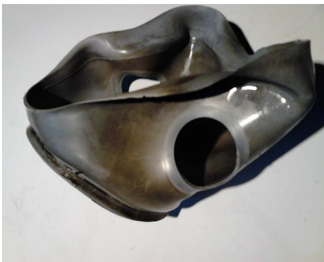
Images 1 and 2. Soot deposits on the inside of the breathing mask after washing in a PPE dishwasher.
