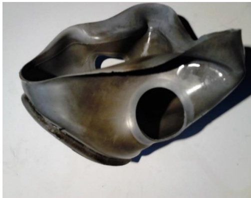
Pictures 5 and 6. Soot and dirt deposits on the insides of breathing masks after cleaning in a PPE dishwasher and not been rinsed manually after cleaning on the inside.
