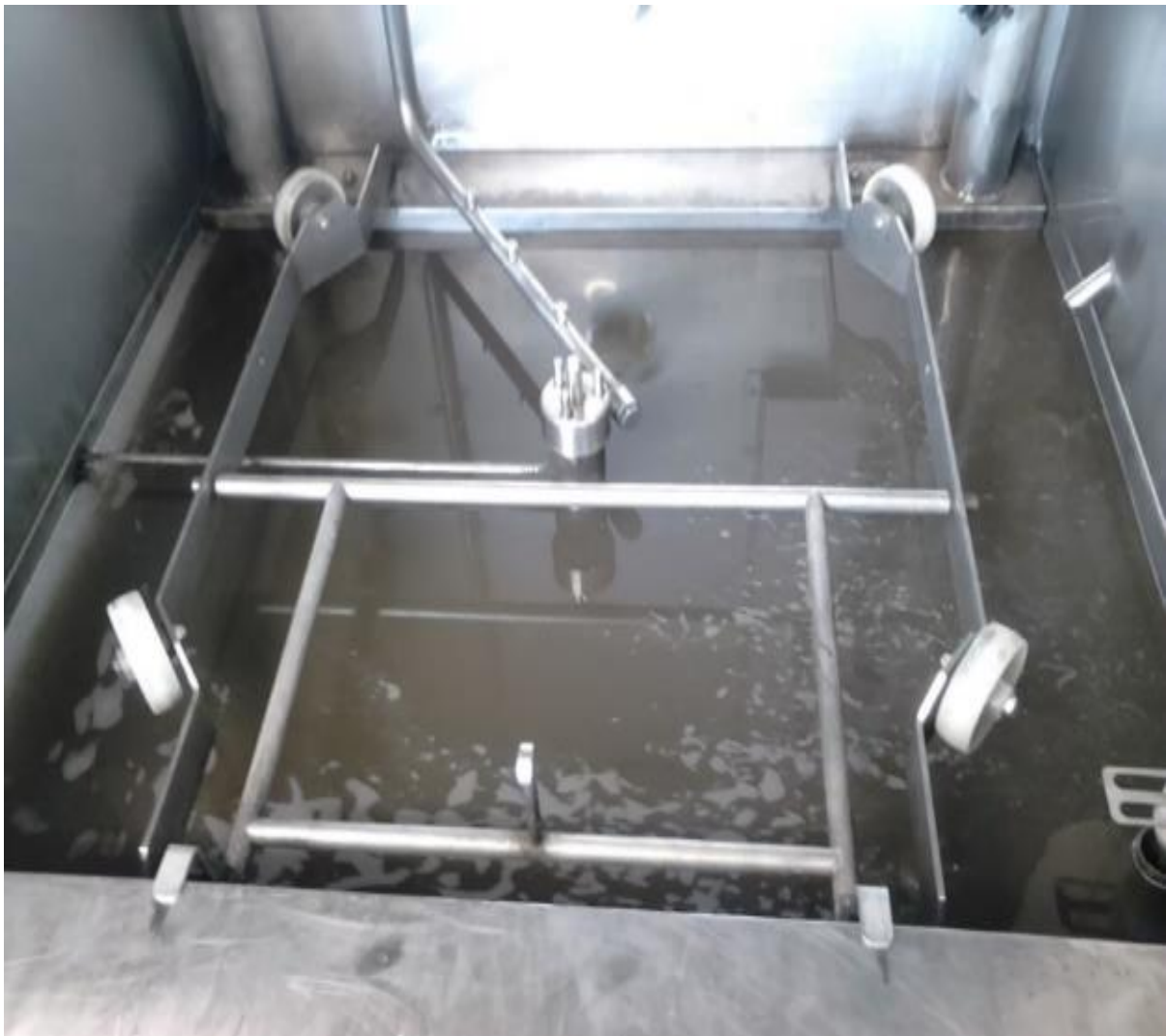
Picture 3. Cleaning water inside a PPE dishwasher contaminated with soot, dirt and hazardous substances after cleaning of breathing apparatus.
