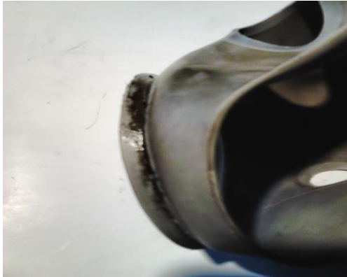
Pictures 5 and 6. Soot and dirt deposits on the insides of breathing masks after cleaning in a PPE dishwasher and not been rinsed manually after cleaning on the inside.
