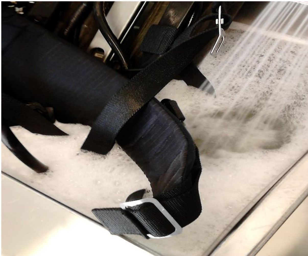
Picture 4. Residues of foaming detergents in carrying harnesses may give rise to heavy foaming when they are cleaned in PPE dishwasher.
