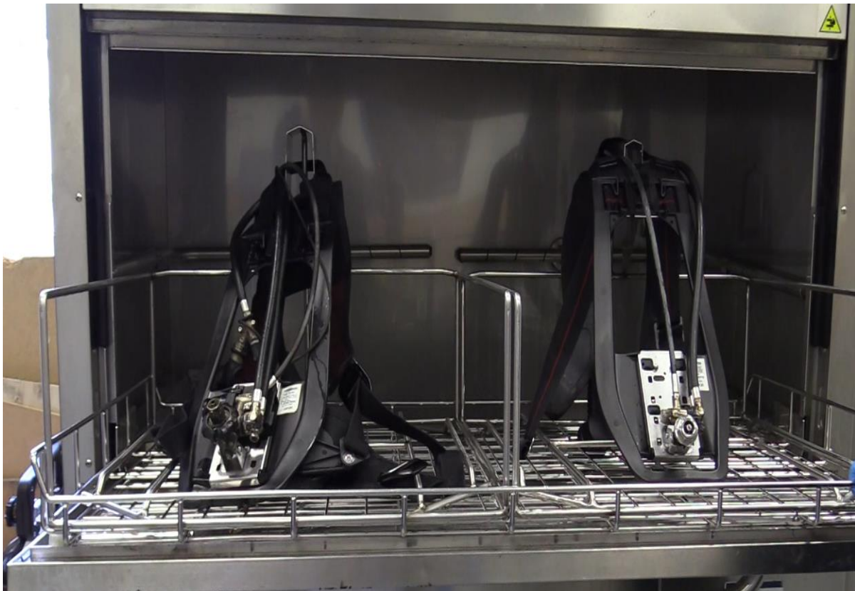
Image 5. Harnesses from breathing apparatus after pre-treatment and washing in a tank washer.
