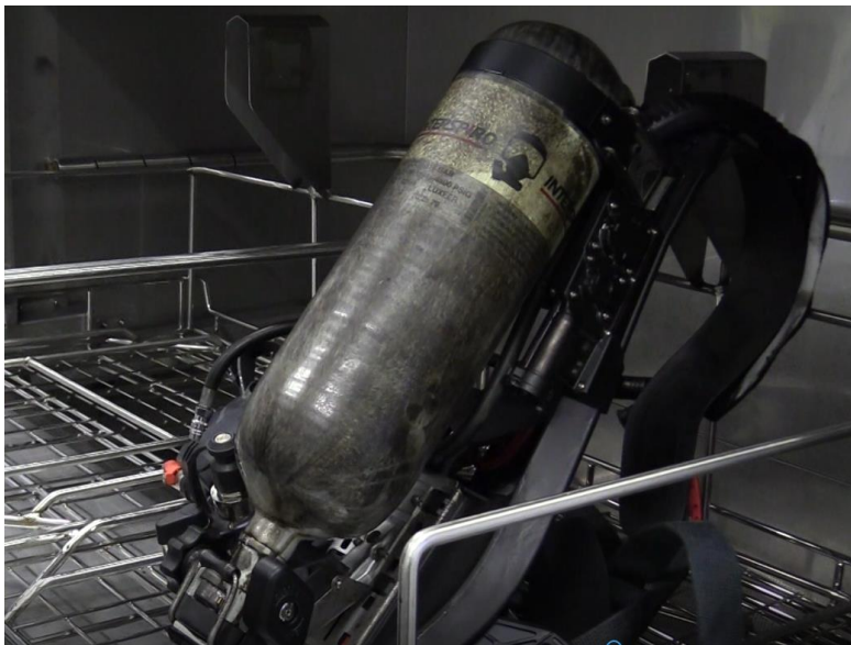
Images 1 and 2. Contaminated and sooty breathing apparatus and parts of the harness before washing
