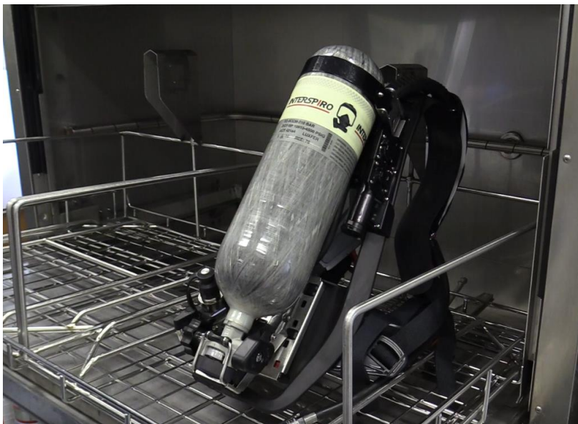
Images 3 and 4. Breathing apparatus and part of a harness from Images 1 and 2 after pre-treatment and washing.
