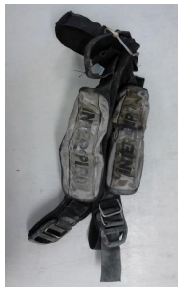
Images 1 and 2. Contaminated and sooty breathing apparatus and parts of the harness before washing
