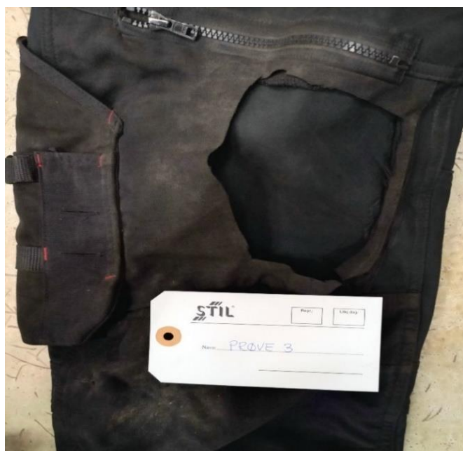
Photo 1. Soot-contaminated trousers, 100% polyester, sampled and analysed for 16 different PAH.
